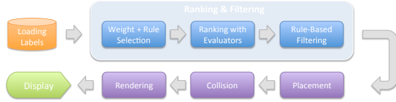
Figure 3: Overview of the entire labeling pipeline: After loading the labels from the map database (orange), the 3-stage filtering system (blue) presented in this paper filters the labels. Then, the selected labels are sent for placement onto the screen (violet). At runtime, we compute if any collision between labels occurs to finally render them to the display (green).
